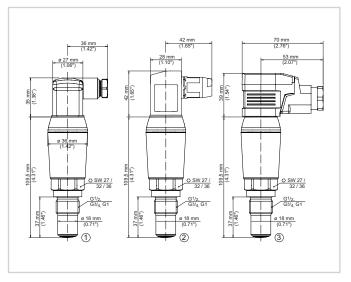
VEGAPOINT 24, standard version - thread with valve plugs acc. to ISO 4400
