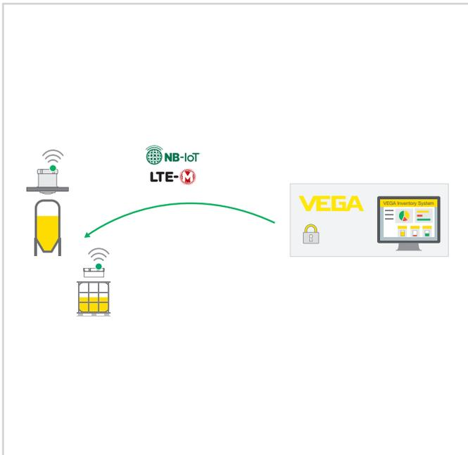
Remote access from VEGA Inventory System via NB-IoT or LTE-M to the sensor
