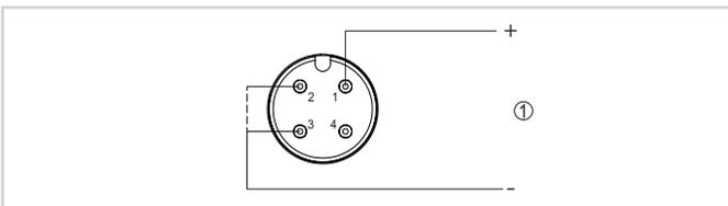
Wiring plan - two-wire 4 ... 20 mA - M12 x 1 plug
