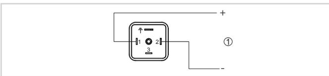
Wiring plan - two-wire 4 ... 20 mA - plug according to ISO 4400
