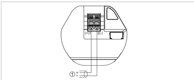
Compartiment de raccordement VEGAPULS 11
