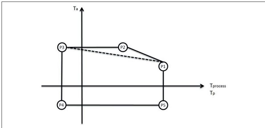
Furthermore it must be observed that the graph defined by the points P1 ... P5 was determined for instruments with a permissible process temperature of up to +195 °C with an isolation (heat conductance of 0.05 W/mK with 2 cm thick insulation). Two layers of insulation material with a thickness of 2 cm each were attached from the tank surface with the mentioned heat conductance.
