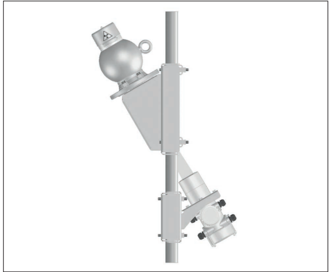
Fig. 7: 30° measurement setup on a pipeline with diameter 50 ... 100 mm (1.97 ... 3.94 in)
