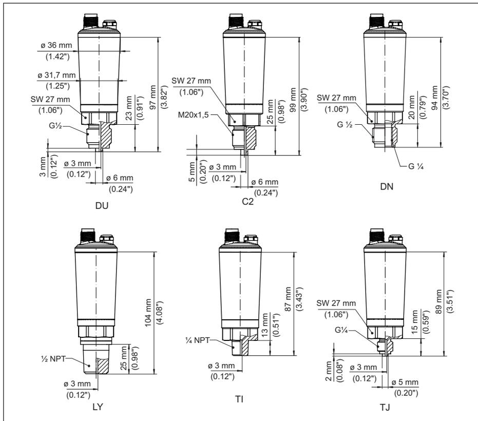
Fig. 31: VEGABAR 29, raccord fileté non arasant
