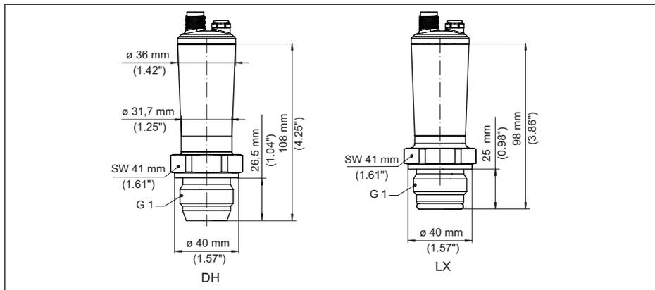
Fig. 33: VEGABAR 29, raccord cône/tube
