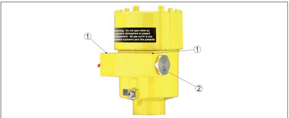
1 Label: Type and size of the thread ½-14 NPT or M20 x 1.5 2 Screw plug
