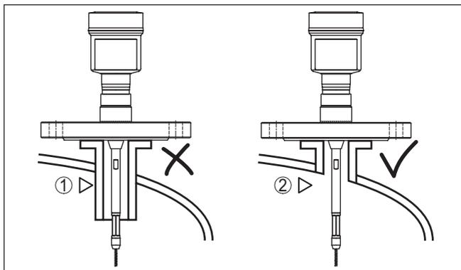
Fig. 6: Montar as luvas de forma nivelada
