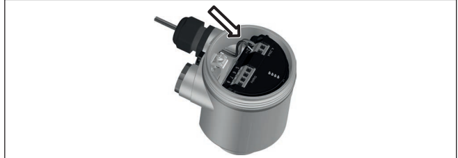
Fig. 7: Connection steps 5 and 6 - Single chamber housing
