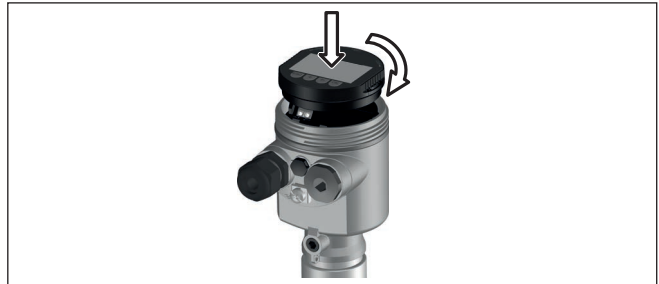
Fig. 6: Installing the display and adjustment module in the electronics compartment of the single chamber housing
