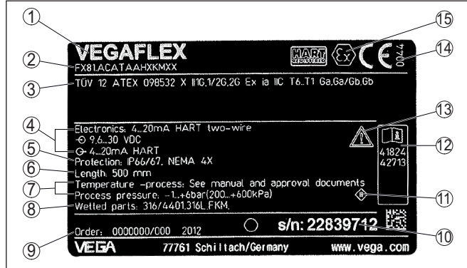
Fig. 1: Layout of the type label (example)
