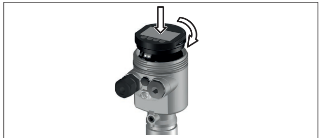
Fig. 9: Installing the display and adjustment module in the electronics compartment of the single chamber housing
