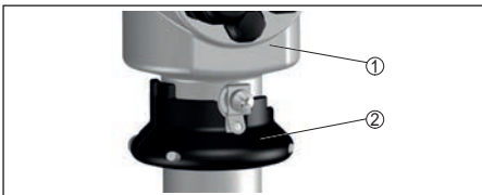
Abb. 12: Housing lock with electropolished stainless steel housing
