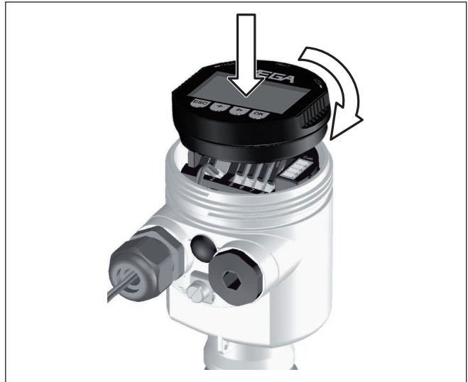
Fig. 6: Insert display and adjustment module in the single chamber housing
