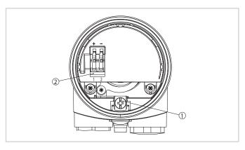
Electronics and terminal compartment, single chamber housing
