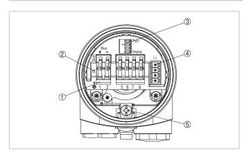
Electronics and terminal compartment, single chamber housing
