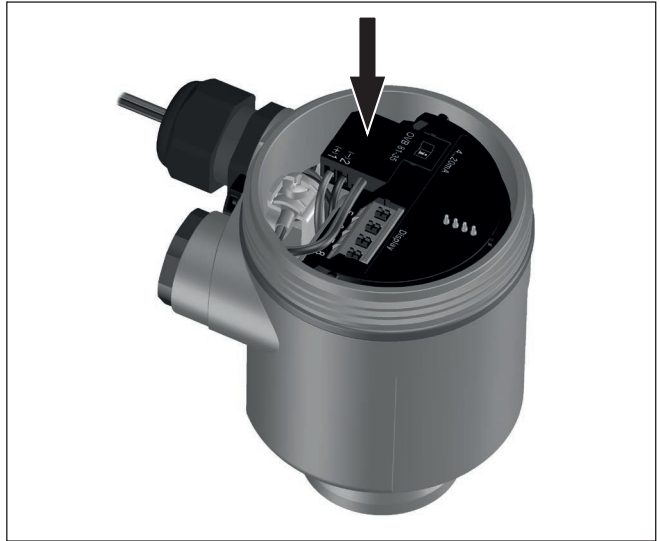
Fig. 2: Plug the overvoltage arrester onto the sensor electronics - single chamber housing
