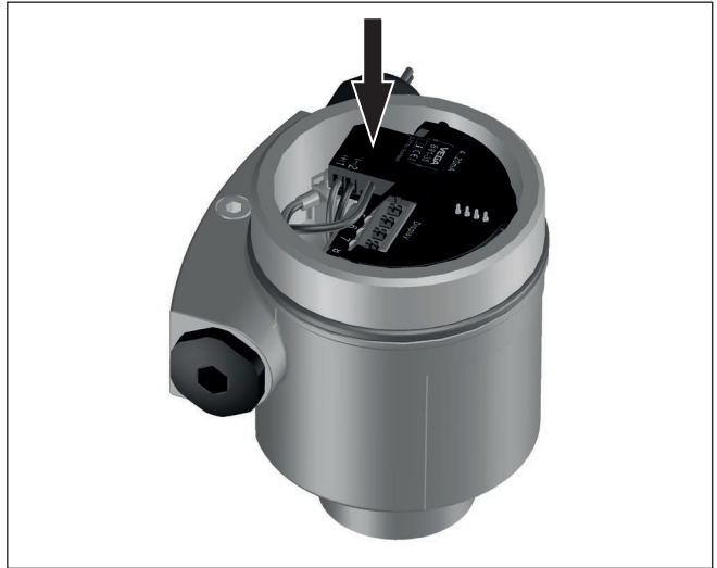
Fig. 3: Plug the overvoltage arrester onto the sensor electronics - Aluminium single chamber housing
