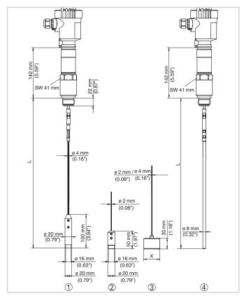
VEGAFLEX 86 - threaded version (-20  $\dots$  +250  $^{\circ}\text{C})$
