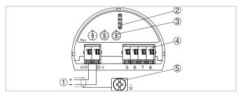
Electronics and terminal compartment, single chamber housing
