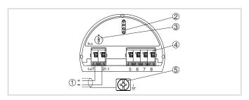
Electronics and connection compartment, single chamber housing
