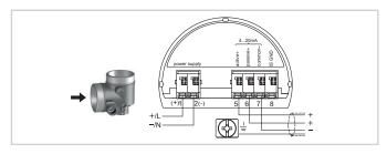
Connection compartment with double chamber housing - low voltage
