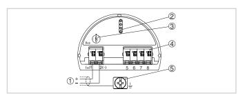
Electronics and terminal compartment, single chamber housing
