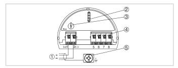
Electronics and terminal compartment, single chamber housing
