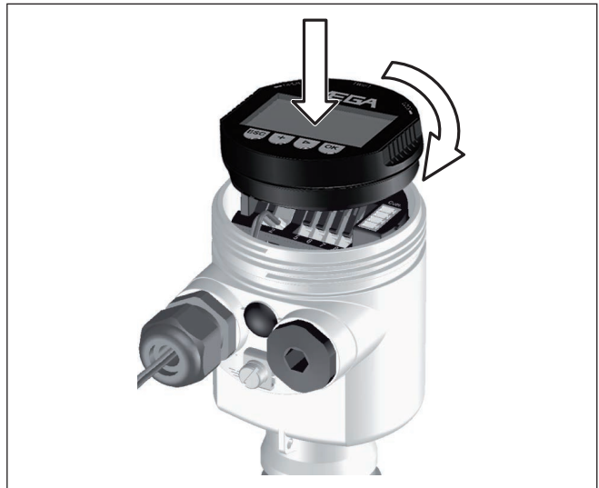
Fig. 20: Insert display and adjustment module in the single chamber housing
